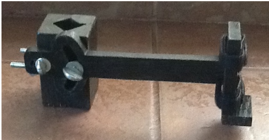
Figure 2 Home-made wheel-chair camera mount
