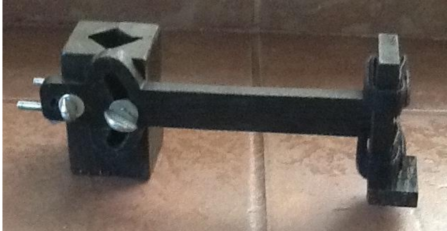
Figure 2 Home-made wheel-chair camera mount
